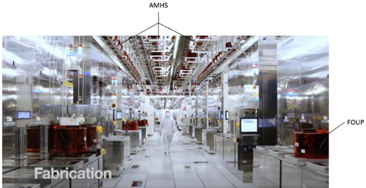
Figure 7: Inside a wafer fab, a worker walks down a row lined with process tools. Wafers are loaded into each tool via FOUPs. An AMHS carries FOUPs throughout the fab to the appropriate tool for processing.
