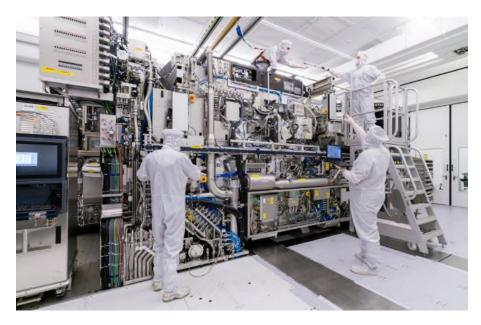
Figure 10-1 ASML Latest Extreme Ultraviolet Photolithography Exposure Tool. 79
