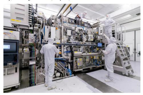
Figure 5: ASML's latest EUV lithography patterning machine (Source: ASML).
