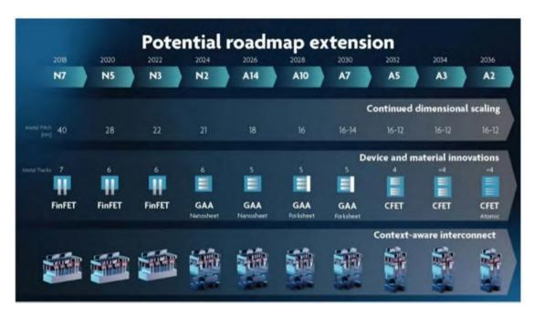
Figure B-4: IMEC's vision of the future logic roadmap, with dimensional scaling predicted to continue through 2036 (IMEC 2023).
